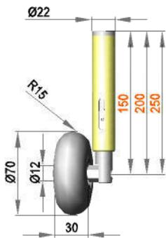
Spring-mounted roller assembly with roller RR12 / 30 / R15 / PO
