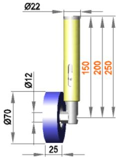
Spring-mounted roller assembly with roller R 12 / 25 / 70 / S50R
