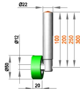
**Fixed roller assembly with roller R 12 / 20 / 50 / AL**
