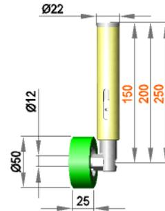
**Spring-mounted roller assembly with roller R 12 / 25 / 50 / AL**
