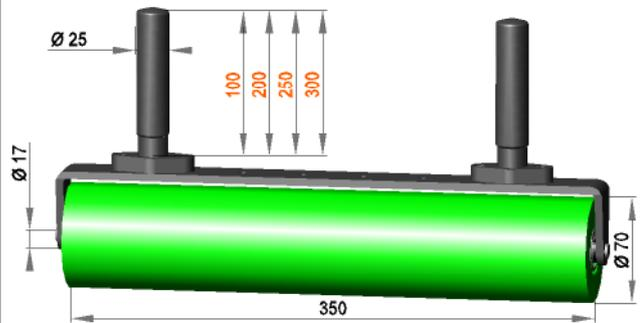
Roller assembly Ø25 with press roller **R 17 / 350 / 70 / AL**
