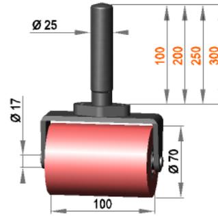
Roller assembly Ø25 with press roller **R 17 / 100 / 70 / S70G**
