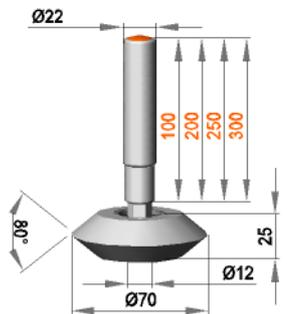
**Fixed holding assembly with roll ER 12 / 25 / 80 / PO**
