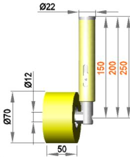
**Spring-mounted roller assembly with roller RB 12 / 50 / 70 / S90Gr**
