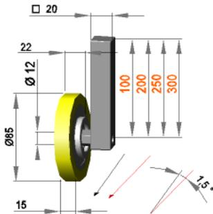
Guide roller assembly 1,5° left with roller F 12 / 15 / 85 / S90Gr
