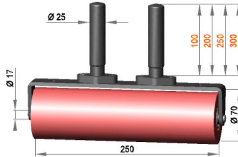
Roller assembly Ø25 with press roller **R 17 / 250 / 70 / S70G**
