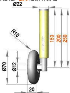
Spring-mounted roller assembly with roller RR12 / 20 / R10 / PO
