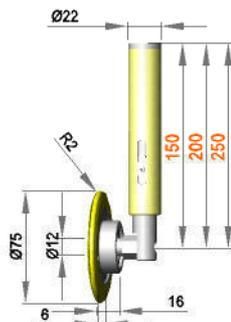
**Spring-mounted roller assembly with roller RRL 12 / 16 / R2 / S90Gr**
