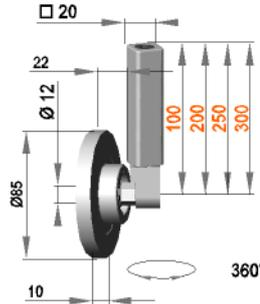
**Swiveling guide roller assembly with roller F 12 / 10 / 85 / PO**
