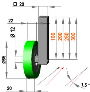
Guide roller assembly 1,5° right with roller F 12 / 20 / 85 / AL
