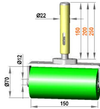
Spring-mounted roller assembly with roller **R 12 / 150 / 70 / AL**
