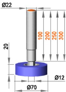
**Fixed roller assembly with roller R 12 / 20 / 70 / S50R**
