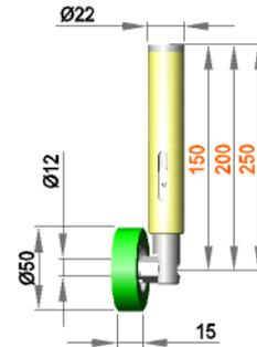
Spring-mounted roller assembly with roller R 12 / 15 / 50 / AL
