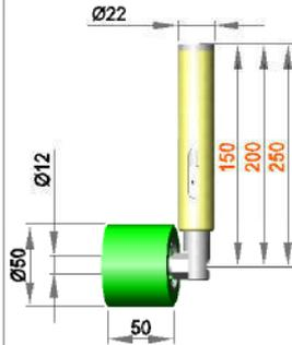
**Spring-mounted roller assembly with roller RB 12 / 50 / 50 / AL**
