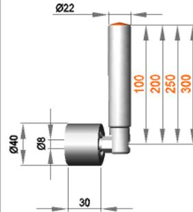
**Fixed roller assembly with roller R 8 / 40 / 40 / S30B**
