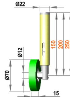
Spring-mounted roller assembly with roller R 12 / 15 / 70 / AL
