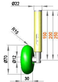
Spring-mounted roller assembly with roller RR12 / 30 / R15 / AL
