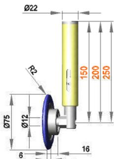
**Spring-mounted roller assembly with roller RRL 12 / 16 / R2 / S50R**
