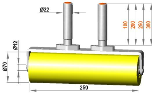
Fixed roller assembly with roller **R 12 / 250 / 70 / S90Gr**
