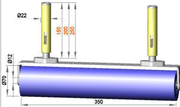
Spring-mounted roller assembly with roller **R 12 / 350 / 70 / S50R**
