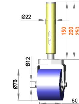
**Spring-mounted roller assembly with roller R 12 / 50 / 70 / S50R**
