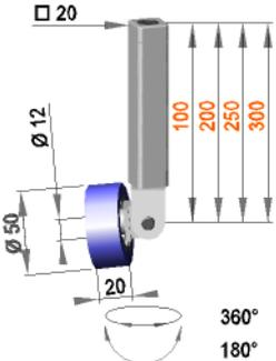
**Universal roller assembly with roller R 12 / 20 / 50 / S50R**
