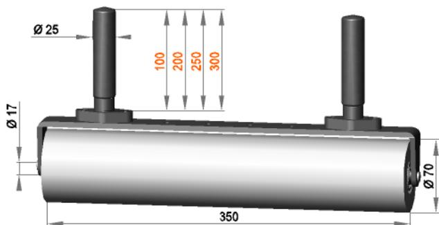
Roller assembly Ø25 with press roller **R 17 / 350 / 70 / PO**
