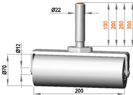
Fixed roller assembly with roller **R 12 / 200 / 70 / PO**
