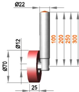
**Fixed roller assembly with roller R 12 / 25 / 70 / S70G**
