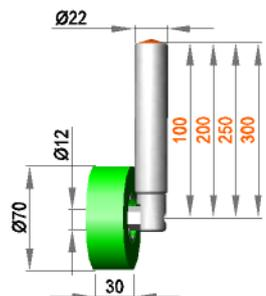
**Fixed roller assembly with roller R 12 / 30 / 70 / AL**
