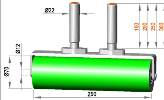
Fixed roller assembly with roller **R 12 / 250 / 70 / AL**
