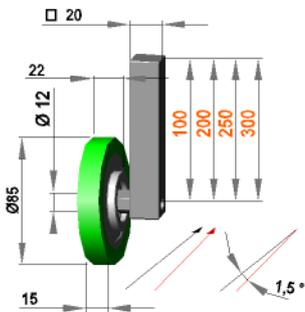
Guide roller assembly 1,5° right with roller F 12 / 15 / 85 / AL
