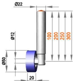
**Fixed roller assembly with roller R 12 / 20 / 50 / S50R**
