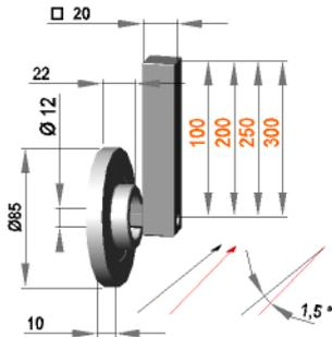
Guide roller assembly 1,5° right with roller F 12 / 10 / 85 / PO
