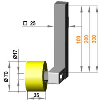
Roller mount □ 25 swiveling with roller R 17 / 35 / 70 / S90Gr
