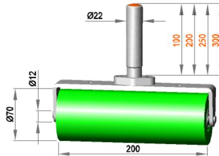
Fixed roller assembly with roller **R 12 / 200 / 70 / AL**
