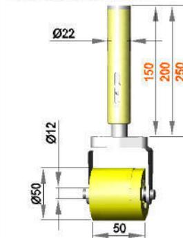
**Spring-mounted roller assembly with roller R 12 / 50 / 50 / S90Gr**
