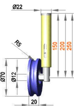
Spring-mounted roller assembly with roller NR12 / 20 / R5 / S50R
