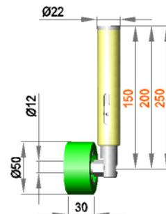
**Spring-mounted roller assembly with roller R 12 / 30 / 50 / AL**
