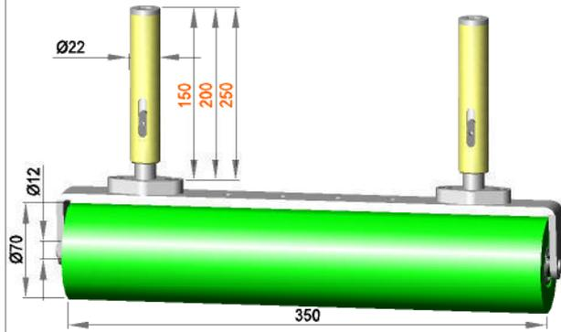
Spring-mounted roller assembly with roller **R 12 / 350 / 70 / AL**
