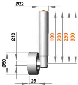
**Fixed roller assembly with roller R 12 / 25 / 50 / PO**
