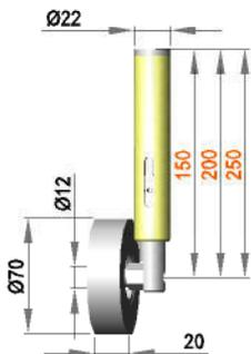
Spring-mounted roller assembly with roller R 12 / 20 / 70 / PO
