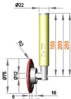
**Spring-mounted roller assembly with roller RRL 12 / 16 / R2 / S70G**
