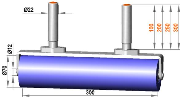
Fixed roller assembly with roller **R 12 / 300 / 70 / S50R**
