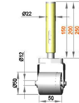
**Spring-mounted roller assembly with roller R 12 / 50 / 50 / PO**
