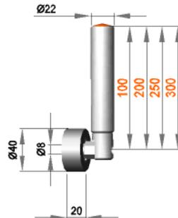
**Fixed roller assembly with roller R 8 / 30 / 40 / S30B**
