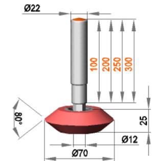
**Fixed roller assembly with roller ER 12 / 25 / 80 / S70G**
