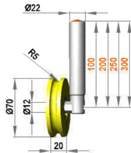
**Fixed roller assembly with roller NR12 / 20 / R5 / S90Gr**
