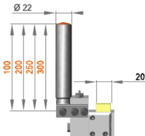
Fixed assembly with felt holder FH/URF/40
