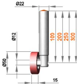
**Fixed roller assembly with roller R 12 / 15 / 50 / S70G**
