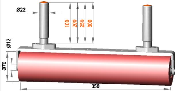
Fixed roller assembly with roller **R 12 / 350 / 70 / S70G**
