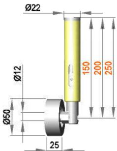
**Spring-mounted roller assembly with roller R 12 / 25 / 50 / PO**
