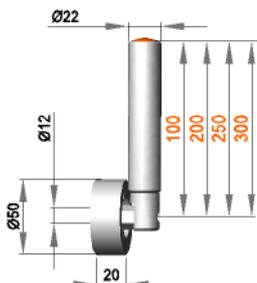
**Fixed roller assembly with roller R 12 / 20 / 50 / PO**
