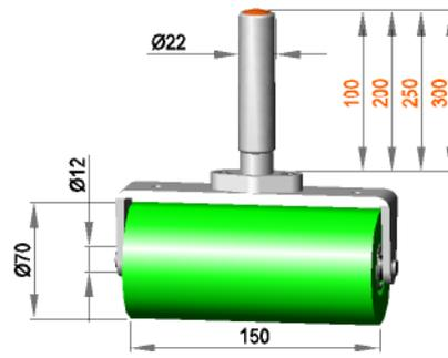
Fixed roller assembly with roller **R 12 / 150 / 70 / AL**
