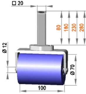
Square roller assembly with roller R 12 / 100 / 70 / S50R
