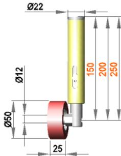
**Spring-mounted roller assembly with roller R 12 / 25 / 50 / S70G**
