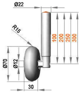
**Fixed holding assembly with roller RR12 / 30 / R15 / PO**
