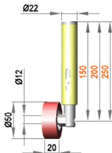
Spring-mounted roller assembly with roller R 12 / 20 / 50 / S70G
