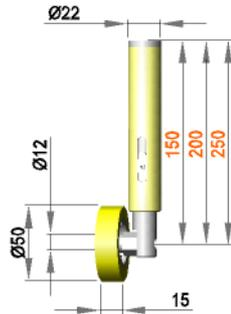
Spring-mounted roller assembly with roller R 12 / 15 / 50 / S90Gr
