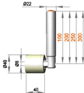
**Fixed roller assembly with roller R 8 / 40 / 40 / ST**
