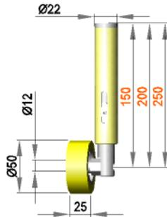
**Spring-mounted roller assembly with roller R 12 / 25 / 50 / S90Gr**
