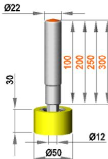
**Fixed roller assembly with roller R 12 / 30 / 50 / S90Gr**
