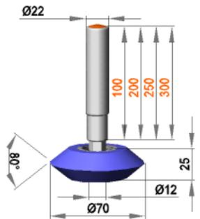
**Fixed roller assembly with roller ER 12 / 25 / 80 / S50R**
