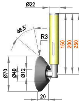
Spring-mounted roller assembly with roller FR12 / 20 / R3 / PO
