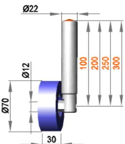
**Fixed roller assembly with roller R 12 / 30 / 70 / S50R**
