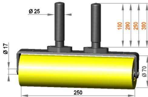
Roller assembly Ø25 with press roller **R 17 / 250 / 70 / S90Gr**
