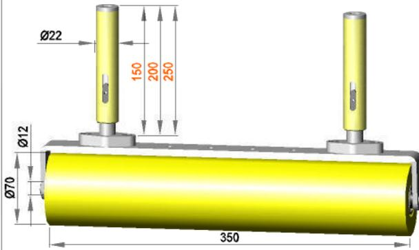
Spring-mounted roller assembly with roller **R 12 / 350 / 70 / S90Gr**
