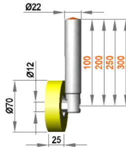
**Fixed roller assembly with roller R 12 / 25 / 70 / S90Gr**
