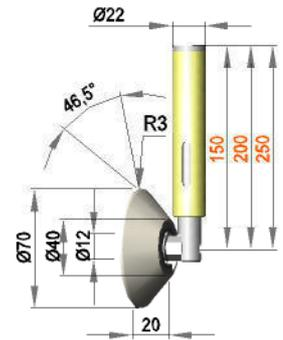
Spring-mounted roller assembly with roller FR12 / 20 / K3 / AL
