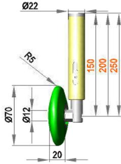
Spring-mounted roller assembly with roller RR12 / 20 / R5 / AL
