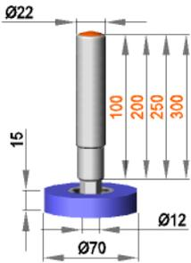
**Fixed roller assembly with roller R 12 / 15 / 70 / S50R**
