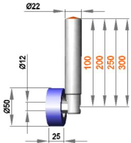
**Fixed roller assembly with roller R 12 / 25 / 50 / S50R**
