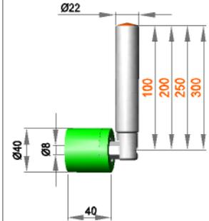
**Fixed roller assembly with roller R 8 / 40 / 40 / AL**
