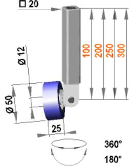
**Universal roller assembly with roller R 12 / 25 / 50 / S50R**
