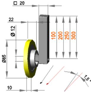
Guide roller assembly 1,5° left with roller F 12 / 10 / 85 / S90Gr
