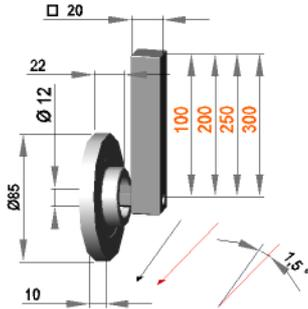
Guide roller assembly 1,5° left with roller F 12 / 10 / 85 / PO
