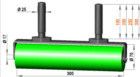
Roller assembly Ø25 with press roller **R 17 / 300 / 70 / AL**
