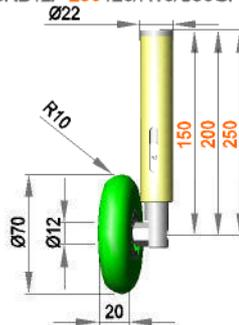
Spring-mounted roller assembly with roller RR12 / 20 / R10 / AL
