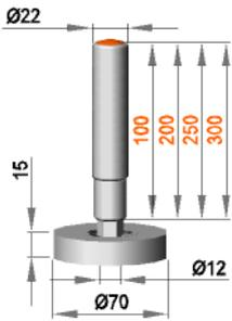
**Fixed roller assembly with roller R 12 / 15 / 70 / PO**
