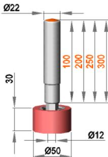
**Fixed roller assembly with roller R 12 / 30 / 50 / S70G**
