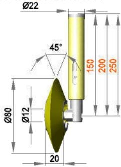
Spring-mounted roller assembly with roller ER 12 / 20 / 45 / S90Gr
