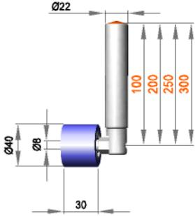
**Fixed roller assembly with roller R 8 / 30 / 40 / S50R**
