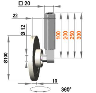
**Universal roller assembly with roller R 12 / 15 / 50 / S30B**
