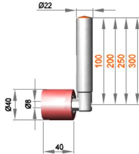
**Fixed roller assembly with roller R 8 / 40 / 40 / S70G**
