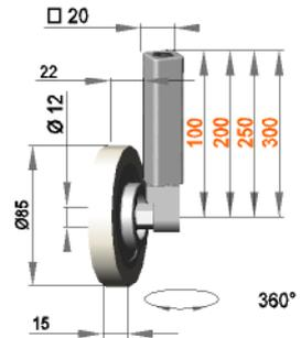
**Swiveling guide roller assembly with roller F 12 / 20 / 85 / S70G**
