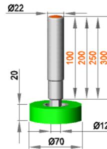
**Fixed roller assembly with roller R 12 / 20 / 70 / AL**
