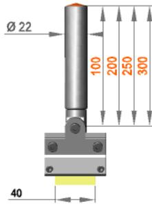
Fixed assembly with felt holder FH/S/60
