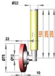
**Spring-mounted roller assembly with roller R 12 / 10 / 75 / S70G**
