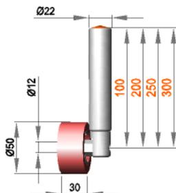
**Fixed roller assembly with roller R 12 / 30 / 50 / S70G**
