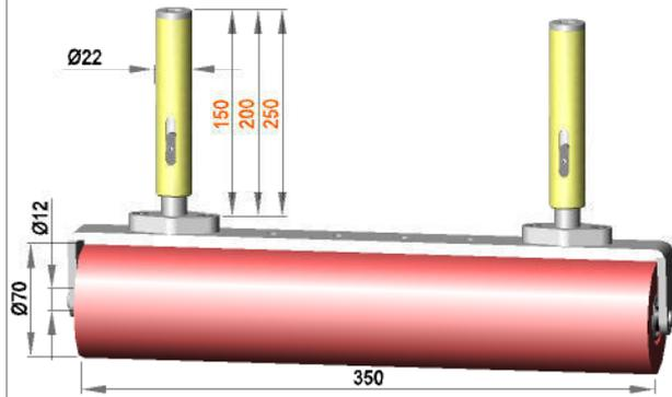
Spring-mounted roller assembly with roller **R 12 / 350 / 70 / S70G**
