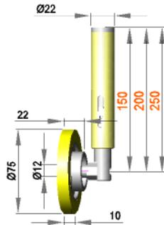
**Spring-mounted roller assembly with roller R 12 / 10 / 75 / S90Gr**
