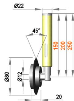
Spring-mounted roller assembly with roller FR12 / 20 / 30 / ST
