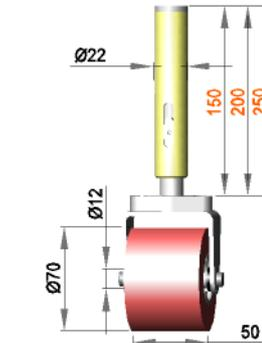
**Spring-mounted roller assembly with roller R 12 / 50 / 70 / S70G**
