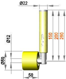
**Spring-mounted roller assembly with roller RB 12 / 50 / 50 / S90Gr**
