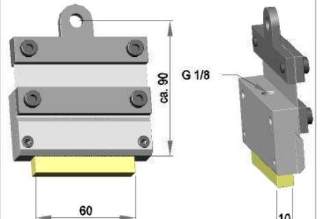
Spring-mounted felt holder, 80mm, mounted top
