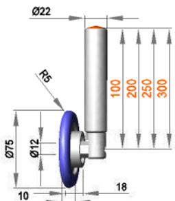
**Fixed roller assembly with roller RRL 12 / 18 / R5 / S50R**
