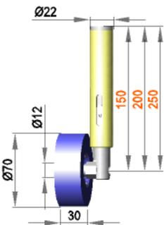
Spring-mounted roller assembly with roller R 12 / 30 / 70 / S50R
