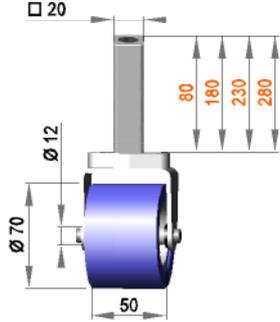
Square roller assembly with roller RB 12 / 50 / 70 / S50R
