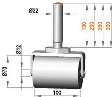
Fixed roller assembly with roller **R 12 / 100 / 70 / PO**
