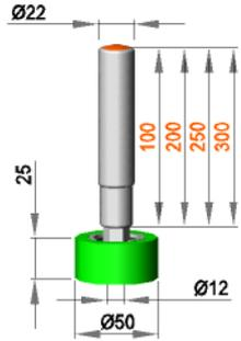
**Fixed roller assembly with roller R 12 / 25 / 50 / AL**
