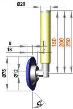
Spring-mounted roller assembly with roller ERL 12 / 18 / L43 / S50R
