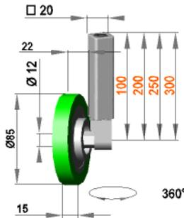
**Swiveling guide roller assembly with roller F 12 / 15 / 85 / AL**
