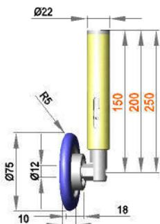
**Spring-mounted roller assembly with roller RRL 12 / 18 / R5 / S50R**
