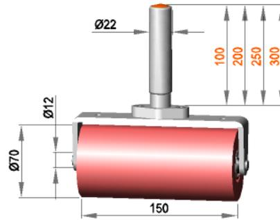
Fixed roller assembly with roller **R 12 / 150 / 70 / S70G**
