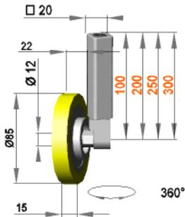
**Swiveling guide roller assembly with roller F 12 / 15 / 85 / S90Gr**
