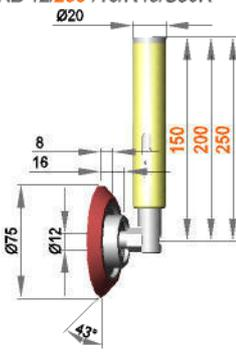
Spring-mounted roller assembly with roller ERL 12 / 16 / R43 / S70G
