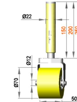
**Spring-mounted roller assembly with roller R 12 / 50 / 70 / S90Gr**
