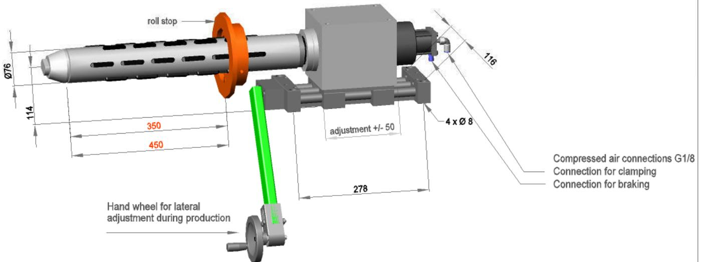
Tension shaft mount with linear guide, bore hole 4x Ø 8 with spacing of 278 x 116.
