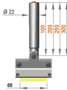
Fixed assembly with felt holder FH/S/80
