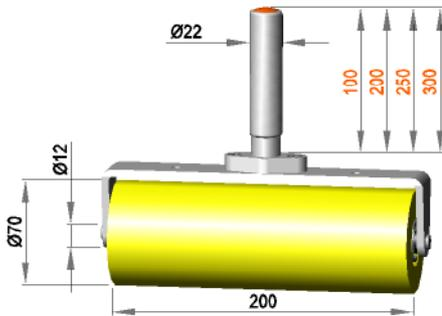
Fixed roller assembly with roller **R 12 / 200 / 70 / S90Gr**
