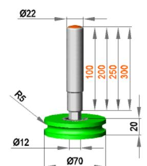
**Fixed holding assembly with roller NR12 / 20 / R5 / AL**
