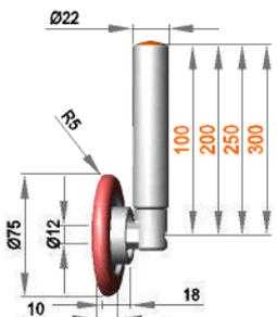
**Fixed roller assembly with roller RRL 12 / 18 / R5 / S70G**
