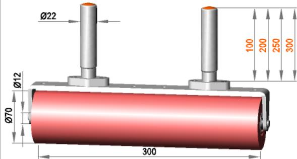
Fixed roller assembly with roller **R 12 / 300 / 70 / S70G**
