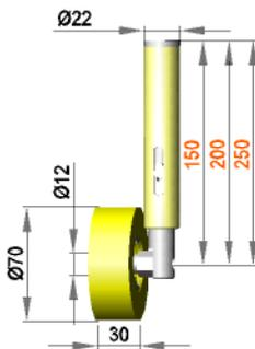
Spring-mounted roller assembly with roller R 12 / 30 / 70 / S90Gr
