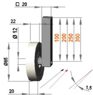
Guide roller assembly 1,5° right with guide roller.
