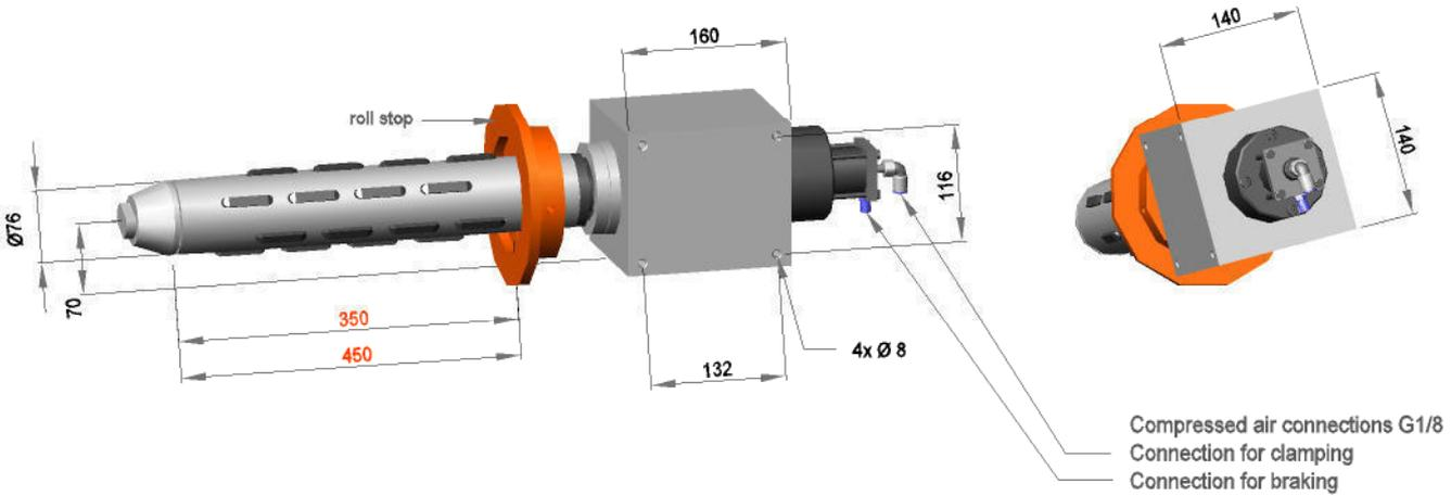
Tension shaft mount is designed for linear guide (132 x 116). Can also be mounted directly
