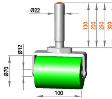
Fixed roller assembly with roller **R 12 / 100 / 70 / AL**
