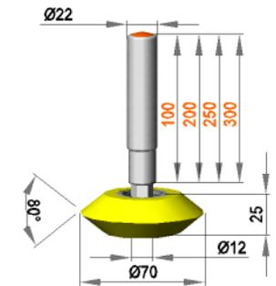
**Fixed roller assembly with roller ER 12 / 25 / 80 / S90Gr**
