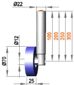
**Fixed roller assembly with roller R 12 / 25 / 70 / S50R**
