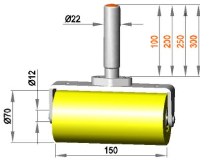
Fixed roller assembly with roller **R 12 / 150 / 70 / S90Gr**
