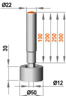
**Fixed roller assembly with roller R 12 / 30 / 50 / PO**
