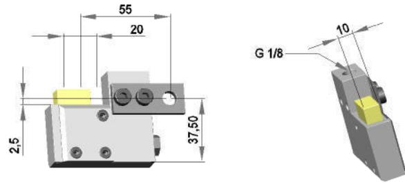
Hose connector, for hoses with an inside diameter of 2mm
