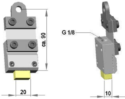
Spring-mounted felt holder, 40mm, mounted top
