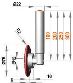
**Fixed roller assembly with roller RRL 12 / 16 / R2 / S70G**
