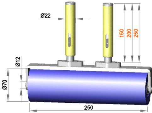
Spring-mounted roller assembly with roller **R 12 / 250 / 70 / S50R**
