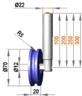
**Fixed roller assembly with roller NR12 / 20 / R5 / S50R**
