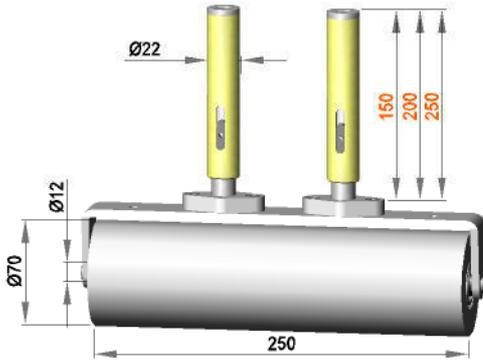
Spring-mounted roller assembly with roller **R 12 / 250 / 70 / PO**
