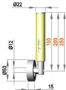
Spring-mounted roller assembly with roller R 12 / 15 / 50 / PO
