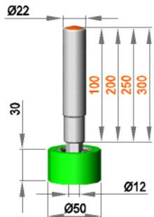
**Fixed roller assembly with roller R 12 / 30 / 50 / AL**
