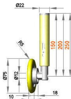
**Spring-mounted roller assembly with roller RRL 12 / 18 / R5 / S90Gr**
