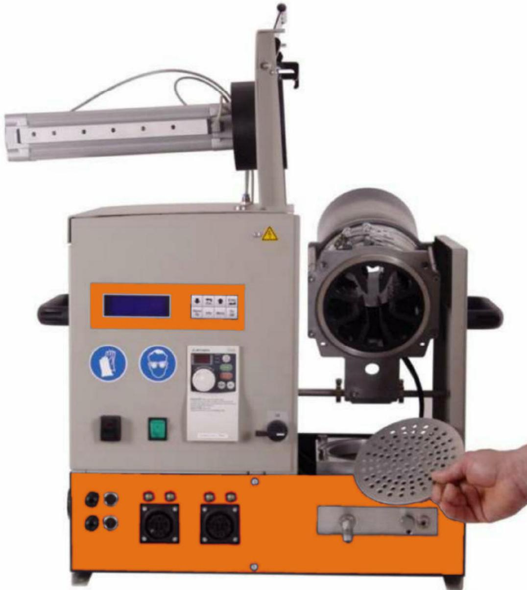
Gluing device ST 920 - GPR/B for 18 - 20 kg foil bags
