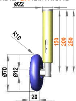
Spring-mounted roller assembly with roller RR12 / 20 / R10 / S50R
