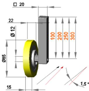
Guide roller assembly 1,5° right with roller F 12 / 15 / 85 / S90Gr
