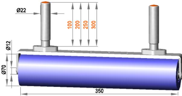
Fixed roller assembly with roller **R 12 / 350 / 70 / S50R**
