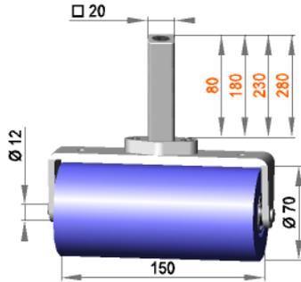
Square roller assembly with roller R 12 / 150 / 70 / S50R
