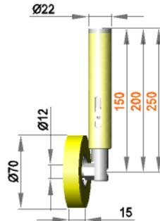
Spring-mounted roller assembly with roller R 12 / 15 / 70 / S90Gr
