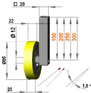
Guide roller assembly 1,5° right with roller F 12 / 20 / 85 / S90Gr
