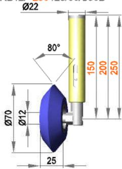
Spring-mounted roller assembly with roller ER 12 / 25 / 80 / S50R
