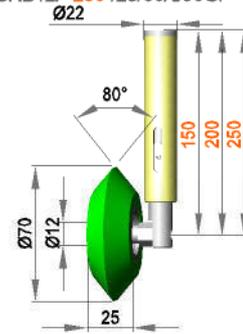
Spring-mounted roller assembly with roll ER 12 / 25 / 80 / AL
