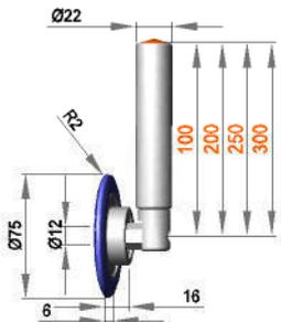
**Fixed roller assembly with roller RRL 12 / 16 / R2 / S50R**
