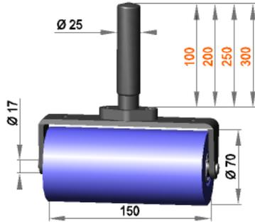
Roller assembly Ø25 with press roller **R 17 / 150 / 70 / S50R**
