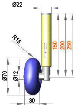
Spring-mounted roller assembly with roller RR12 / 30 / R15 / S50R
