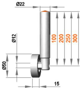
**Fixed roller assembly with roller R 12 / 15 / 50 / PO**
