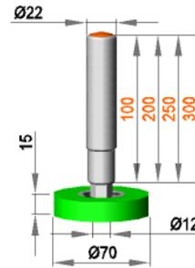
**Fixed roller assembly with roller R 12 / 15 / 70 / AL**
