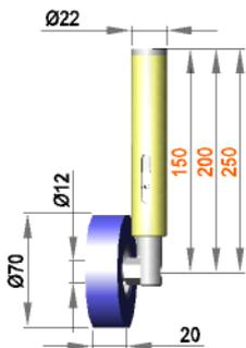
Spring-mounted roller assembly with roller R 12 / 20 / 70 / S50R
