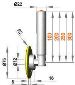
**Fixed roller assembly with roller RRL 12 / 16 / R2 / S90Gr**
