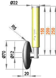
Spring-mounted roller assembly with roller RR12 / 20 / R5 / PO
