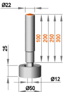
**Fixed roller assembly with roller R 12 / 25 / 50 / PO**
