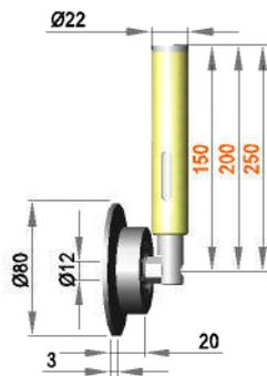
Spring-mounted roller assembly with roller FR12 / 20 / 45 / AL
