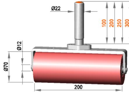
Fixed roller assembly with roller **R 12 / 200 / 70 / S70G**
