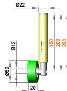
Spring-mounted roller assembly with roller R 12 / 20 / 50 / AL
