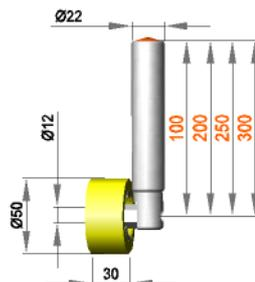
**Fixed roller assembly with roller R 12 / 30 / 50 / S90Gr**
