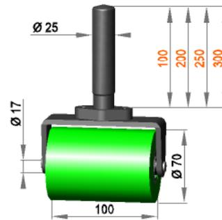
Roller assembly Ø25 with press roller **R 17 / 100 / 70 / AL**
