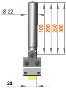
Fixed assembly with felt holder FH/S/40
