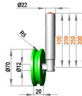
**Fixed holding assembly with roller NR12 / 20 / R5 / AL**
