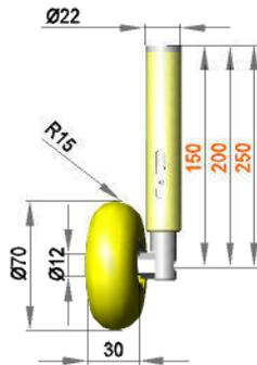
Spring-mounted roller assembly with roller RR12 / 30 / R15 / S90Gr
