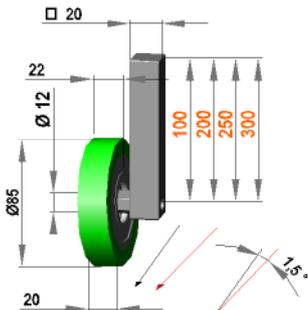
Guide roller assembly 1,5° left with roller F 12 / 20 / 85 / AL
