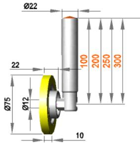
**Fixed roller assembly with roller R 12 / 10 / 75 / S90Gr**
