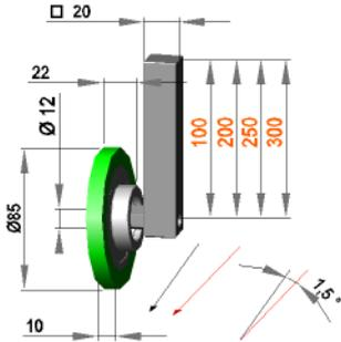
Guide roller assembly 1,5° left with roller F 12 / 10 / 85 / AL
