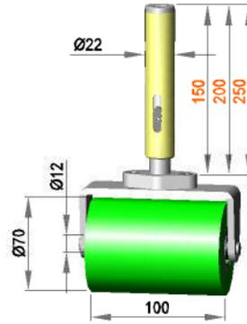
Spring-mounted roller assembly with roller **R 12 / 100 / 70 / AL**
