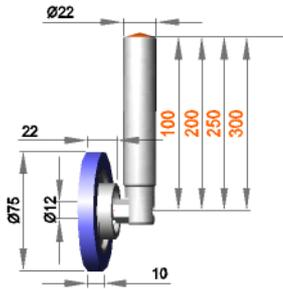
**Fixed roller assembly with roller R 12 / 10 / 75 / S50R**
