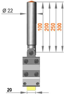
Fixed assembly with felt holder FH/G/40
