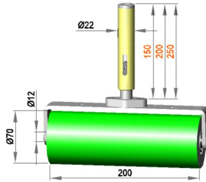
Spring-mounted roller assembly with roller **R 12 / 200 / 70 / AL**
