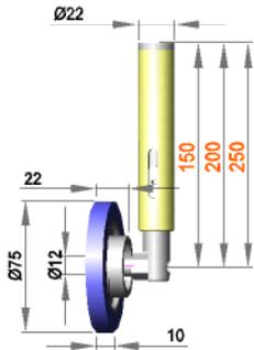
**Spring-mounted roller assembly with roller R 12 / 10 / 75 / S50R**
