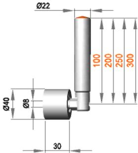
**Fixed roller assembly with roller R 8 / 30 / 40 / SK**
