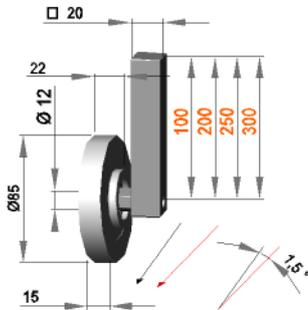
Guide roller assembly 1,5° left with roller F 12 / 15 / 85 / PO
