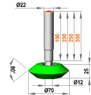
**Fixed holding assembly with roll ER 12 / 25 / 80 / AL**
