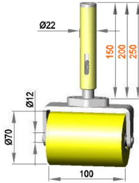
Spring-mounted roller assembly with roller **R 12 / 100 / 70 / S90Gr**
