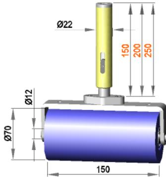
Spring-mounted roller assembly with roller **R 12 / 150 / 70 / S50R**
