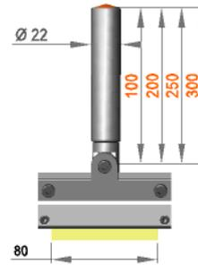
Fixed assembly with felt holder FH/S/100
