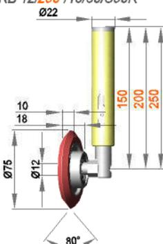
Spring-mounted roller assembly with roller ERL 12 / 18 / 80 / S70G
