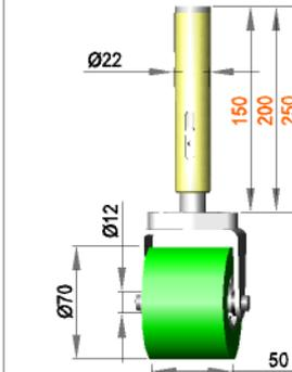
**Spring-mounted roller assembly with roller R 12 / 50 / 70 / AL**
