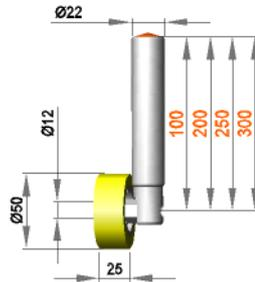
**Fixed roller assembly with roller R 12 / 25 / 50 / S90Gr**
