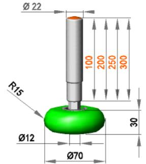
**Fixed holding assembly with roller RR12 / 30 / R15 / AL**
