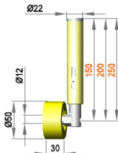
**Spring-mounted roller assembly with roller R 12 / 30 / 50 / S90Gr**
