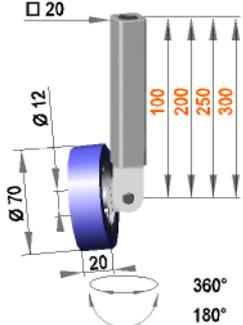
**Universal roller assembly with roller R 12 / 20 / 70 / S50R**
