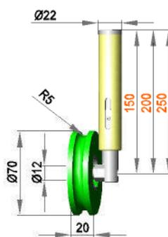
Spring-mounted roller assembly with roller NR12 / 20 / R5 / AL
