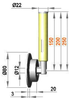
Spring-mounted roller assembly with roller FR12 / 20 / K3 / PO
