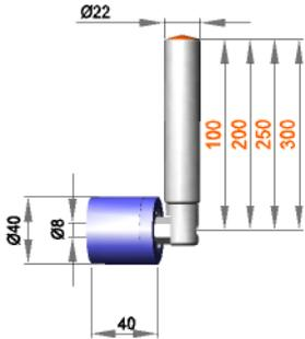
**Fixed roller assembly with roller R 8 / 40 / 40 / S50R**
