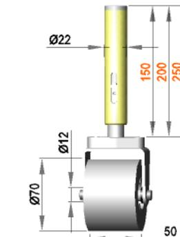
**Spring-mounted roller assembly with roller R 12 / 50 / 70 / PO**
