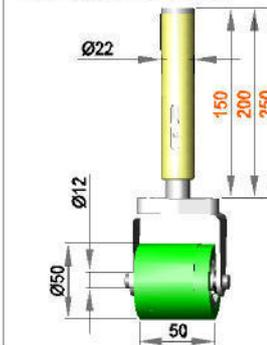
**Spring-mounted roller assembly with roller R 12 / 50 / 50 / AL**
