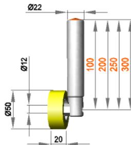
**Fixed roller assembly with roller R 12 / 20 / 50 / S90Gr**
