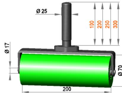
Roller assembly Ø25 with press roller **R 17 / 200 / 70 / AL**
