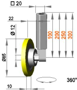
**Swiveling guide roller assembly with roller F 12 / 10 / 85 / S90Gr**
