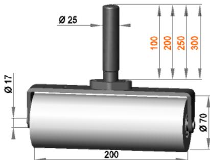
Roller assembly Ø25 with press roller **R 17 / 200 / 70 / PO**
