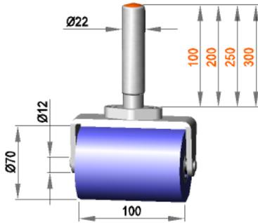
Fixed roller assembly with roller **R 12 / 100 / 70 / S50R**
