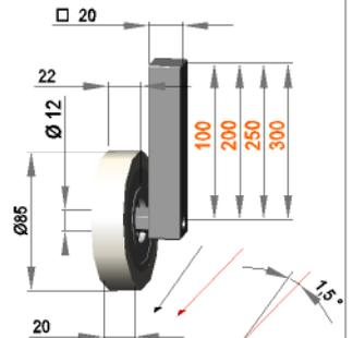
Guide roller assembly 1,5° left with guide roller.
