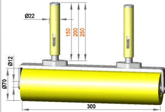
Spring-mounted roller assembly with roller **R 12 / 300 / 70 / S90Gr**
