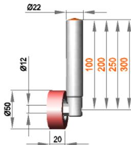
**Fixed roller assembly with roller R 12 / 20 / 50 / S70G**
