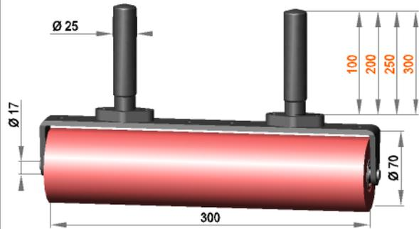
Roller assembly Ø25 with press roller **R 17 / 300 / 70 / S70G**
