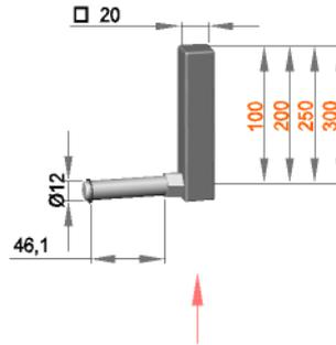
The low gradient of 1.5° set the guide roller obliquely. So the profile is pressed with slight pressure. **This left version must be arranged with the right version.**
