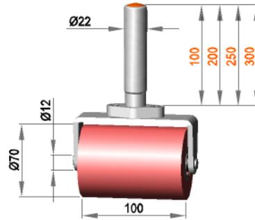
Fixed roller assembly with roller **R 12 / 100 / 70 / S70G**
