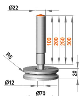
**Fixed holding assembly with roller NR12 / 20 / R5 / PO**
