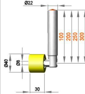
**Fixed roller assembly with roller R 8 / 30 / 40 / S90Gr**
