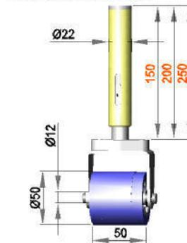
**Spring-mounted roller assembly with roller R 12 / 50 / 50 / S50R**
