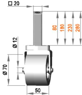
Square roller assembly with roller RB 12 / 50 / 70 / PO
