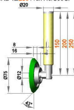
Spring-mounted roller assembly with roller ERL 12 / 16 / 45 / S30B
