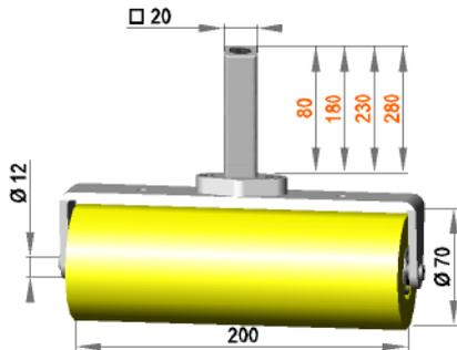
Square roller assembly with roller R 12 / 200 / 70 / S90Gr
