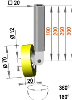
**Universal roller assembly with roller R 12 / 20 / 70 / S90Gr**
