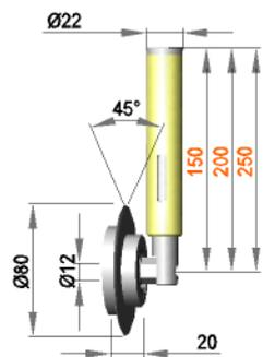
Spring-mounted roller assembly with roller FR12 / 20 / 45 / PO
