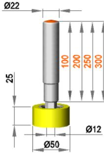
**Fixed roller assembly with roller R 12 / 25 / 50 / S90Gr**
