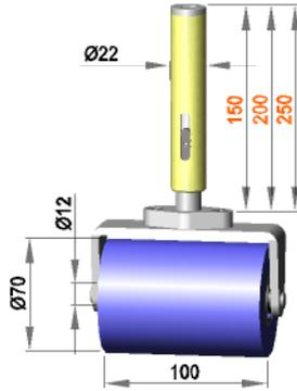
Spring-mounted roller assembly with roller **R 12 / 100 / 70 / S50R**
