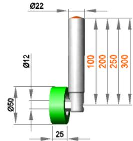
**Fixed roller assembly with roller R 12 / 25 / 50 / AL**
