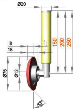
Spring-mounted roller assembly with roller ERL 12 / 18 / L43 / S70G
