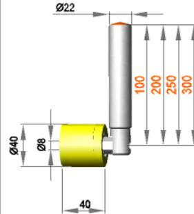
**Fixed roller assembly with roller R 8 / 40 / 40 / S90Gr**
