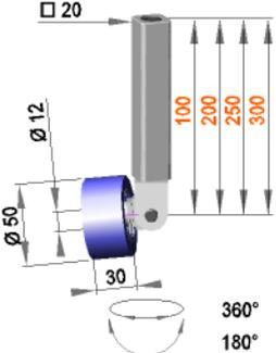
**Universal roller assembly with roller R 12 / 30 / 50 / S50R**
