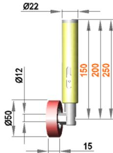
Spring-mounted roller assembly with roller R 12 / 15 / 50 / S70G
