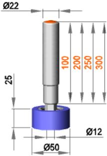
**Fixed roller assembly with roller R 12 / 25 / 50 / S50R**
