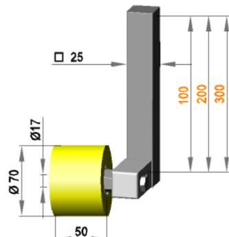
Roller mount □ 25 swiveling with roller R 17 / 50 / 70 / S90Gr
