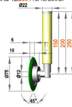
Spring-mounted roller assembly with roller ERL 12 / 18 / 80 / S30B
