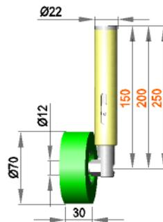
Spring-mounted roller assembly with roller R 12 / 30 / 70 / AL
