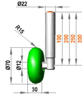
**Fixed holding assembly with roller RR12 / 30 / R15 / AL**
