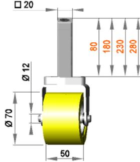
Square roller assembly with roller RB 12 / 50 / 70 / S90Gr
