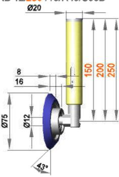
Spring-mounted roller assembly with roller ERL 12 / 16 / R43 / S50R
