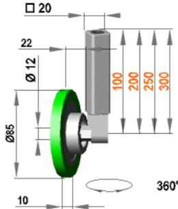
**Swiveling guide roller assembly with roller F 12 / 10 / 85 / AL**
