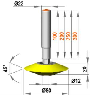
**Fixed roller assembly with roller ER 12 / 20 / 45 / S90Gr**
