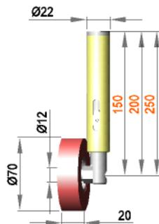
Spring-mounted roller assembly with roller R 12 / 20 / 70 / S70G
