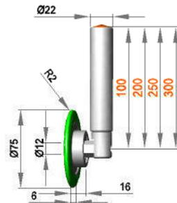
**Fixed roller assembly with roller RRL 12 / 18 / R5 / S30B**
