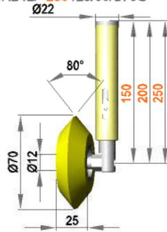
Spring-mounted roller assembly with roller ER 12 / 25 / 80 / S90Gr
