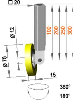
**Universal roller assembly with roller R 12 / 15 / 70 / S90Gr**
