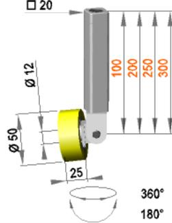
**Universal roller assembly with roller R 12 / 25 / 50 / S90Gr**
