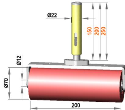
Spring-mounted roller assembly with roller **R 12 / 200 / 70 / S70G**
