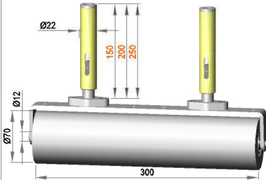
Spring-mounted roller assembly with roller **R 12 / 300 / 70 / PO**
