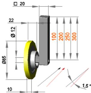
Guide roller assembly 1,5° right with roller F 12 / 10 / 85 / S90Gr
