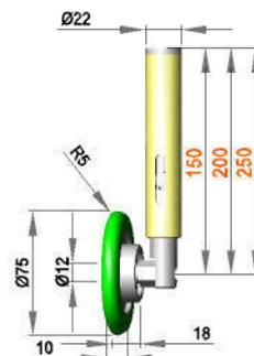
Spring-mounted roller assembly with roller ERL 12 / 18 / L43 / S30B
