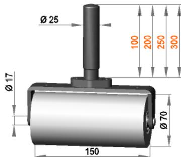
Roller assembly Ø25 with press roller **R 17 / 150 / 70 / PO**
