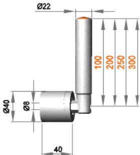
**Fixed roller assembly with roller R 8 / 40 / 40 / SK**
