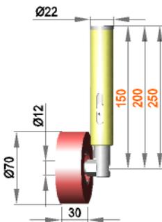
Spring-mounted roller assembly with roller R 12 / 30 / 70 / S70G
