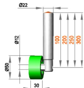
**Fixed roller assembly with roller R 12 / 30 / 50 / AL**
