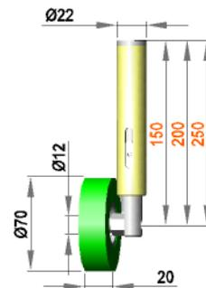
Spring-mounted roller assembly with roller R 12 / 20 / 70 / AL
