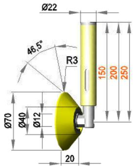
Spring-mounted roller assembly with roller FR12 / 20 / R3 / S90Gr
