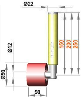
**Spring-mounted roller assembly with roller RB 12 / 50 / 50 / S70G**
