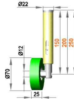
Spring-mounted roller assembly with roller R 12 / 25 / 70 / AL
