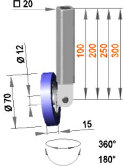
**Universal roller assembly with roller R 12 / 15 / 70 / S50R**
