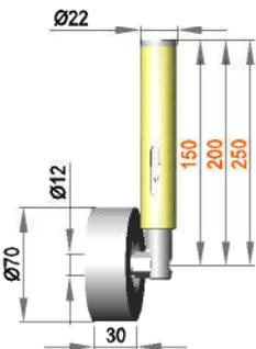
Spring-mounted roller assembly with roller R 12 / 30 / 70 / PO
