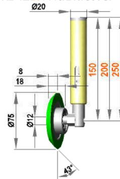
Spring-mounted roller assembly with roller ERL 12 / 16 / R43 / S30B
