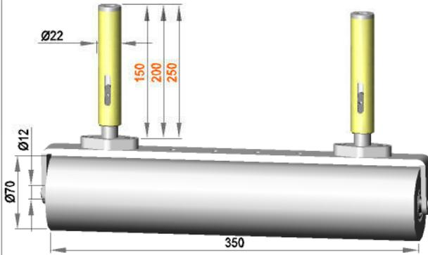
Spring-mounted roller assembly with roller **R 12 / 350 / 70 / PO**
