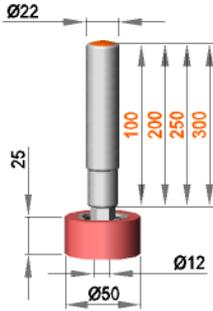
**Fixed roller assembly with roller R 12 / 25 / 50 / S70G**
