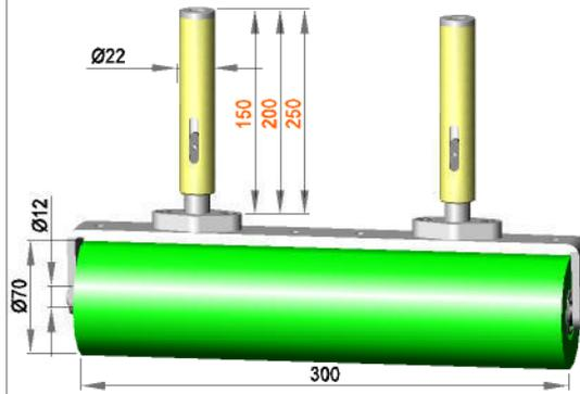
Spring-mounted roller assembly with roller **R 12 / 300 / 70 / AL**
