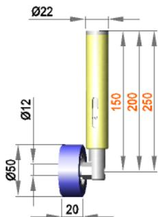
Spring-mounted roller assembly with roller R 12 / 20 / 50 / S50R
