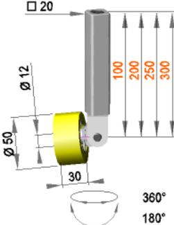
**Universal roller assembly with roller R 12 / 30 / 50 / S90Gr**
