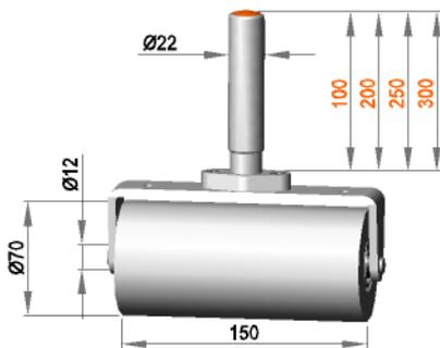
Fixed roller assembly with roller **R 12 / 150 / 70 / PO**
