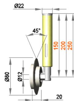
Spring-mounted roller assembly with roller FR12 / 20 / 45 / ST
