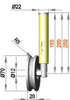
Spring-mounted roller assembly with roller NR12 / 20 / R5 / PO
