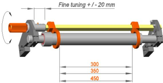
Foil controller with manual width adjustment and fine adjustment
