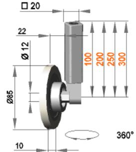
**Swiveling guide roller assembly with roller F 12 / 15 / 85 / S70G**
