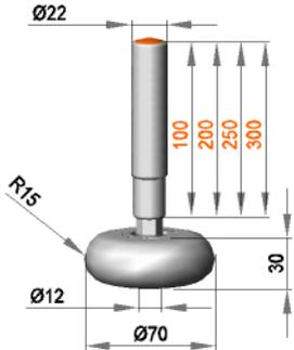
**Fixed holding assembly with roller RR12 / 30 / R15 / PO**
