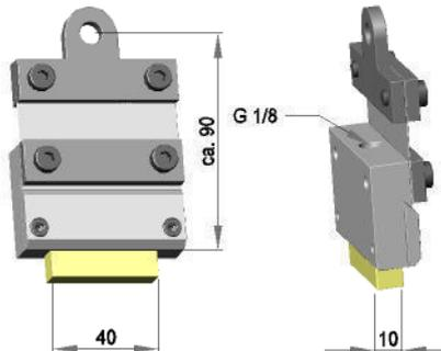
Spring-mounted felt holder, 60mm, mounted top
