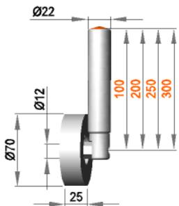
**Fixed roller assembly with roller R 12 / 25 / 70 / PO**
