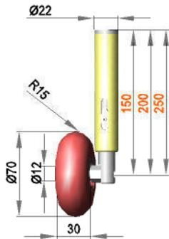
Spring-mounted roller assembly with roller RR12 / 30 / R15 / S70G
