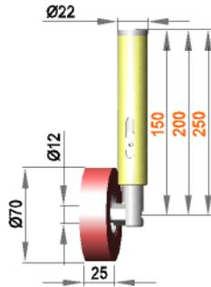
Spring-mounted roller assembly with roller R 12 / 25 / 70 / S70G
