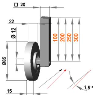
Guide roller assembly 1,5° right with roller F 12 / 15 / 85 / PO
