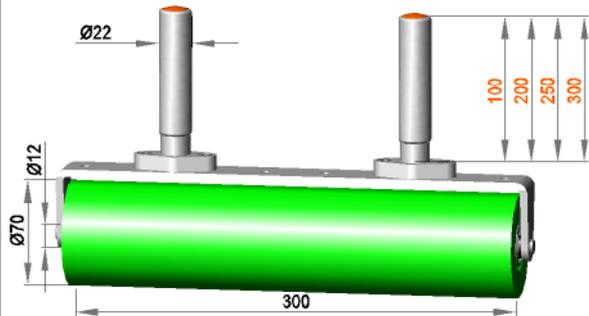
Fixed roller assembly with roller **R 12 / 300 / 70 / AL**
