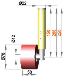
**Spring-mounted roller assembly with roller RB 12 / 50 / 70 / S70G**
