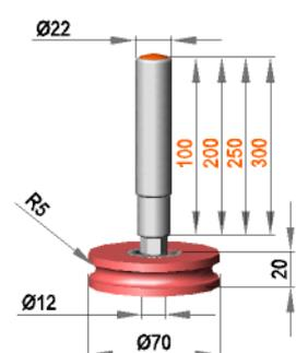
**Fixed roller assembly with roller NR12 / 20 / R5 / S70G**
