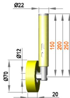
Spring-mounted roller assembly with roller R 12 / 20 / 70 / S90Gr
