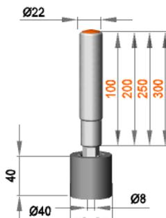
Spring-mounted roller assembly with roller R 12 / 15 / 50 / S30B
