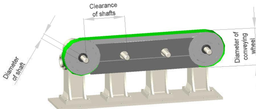
*Machine frame, drive assembly not included in scope of delivery.*
