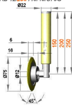
Spring-mounted roller assembly with roller ERL 12 / 16 / 45 / S90Gr
