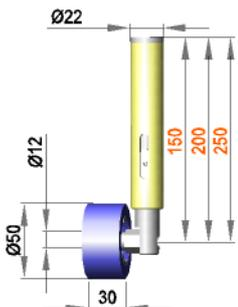
**Spring-mounted roller assembly with roller R 12 / 30 / 50 / S50R**
