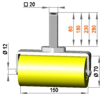
Square roller assembly with roller R 12 / 150 / 70 / S90Gr
