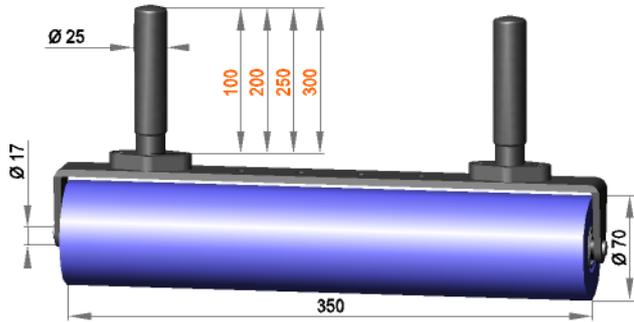
Roller assembly Ø25 with press roller **R 17 / 350 / 70 / S50R**
