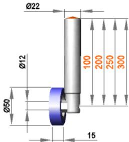
**Fixed roller assembly with roller R 12 / 15 / 50 / S50R**
