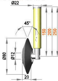
Spring-mounted roller assembly with roller ER 12 / 20 / 45 / PO
