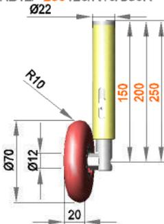
Spring-mounted roller assembly with roller RR12 / 20 / R10 / S70G
