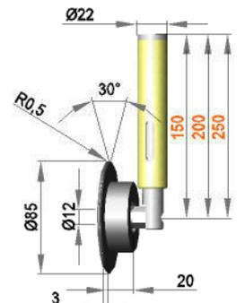
Spring-mounted roller assembly with roller FR12 / 20 / 30 / VA
