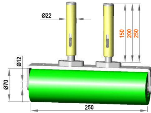
Spring-mounted roller assembly with roller **R 12 / 250 / 70 / AL**
