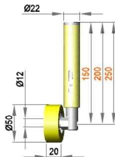
Spring-mounted roller assembly with roller R 12 / 20 / 50 / S90Gr
