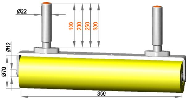
Fixed roller assembly with roller **R 12 / 350 / 70 / S90Gr**
