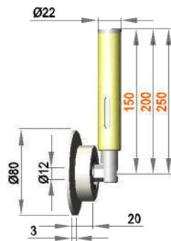
Spring-mounted roller assembly with roller FR12 / 20 / K3 / ST
