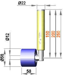
**Spring-mounted roller assembly with roller RB 12 / 50 / 50 / S50R**
