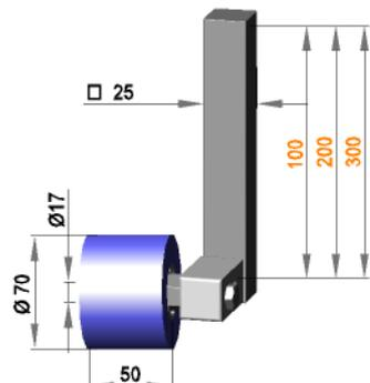
Roller mount □ 25 swiveling with roller R 17 / 50 / 70 / S50R
