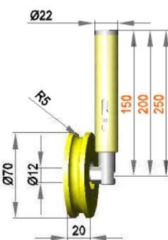
Spring-mounted roller assembly with roller NR12 / 20 / R5 / S90Gr
