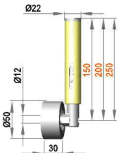
**Spring-mounted roller assembly with roller R 12 / 30 / 50 / PO**
