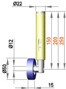
Spring-mounted roller assembly with roller R 12 / 15 / 50 / S50R
