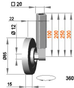
**Swiveling guide roller assembly with roller F 12 / 15 / 85 / PO**
