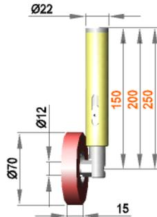
Spring-mounted roller assembly with roller R 12 / 15 / 70 / S70G
