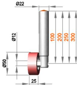
**Fixed roller assembly with roller R 12 / 25 / 50 / S70G**
