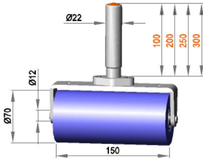
Fixed roller assembly with roller **R 12 / 150 / 70 / S50R**
