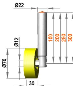
**Fixed roller assembly with roller R 12 / 30 / 70 / S90Gr**
