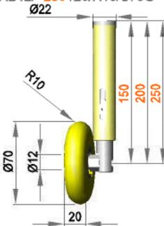
Spring-mounted roller assembly with roller RR12 / 20 / R10 / S90Gr
