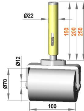
Spring-mounted roller assembly with roller **R 12 / 100 / 70 / PO**
