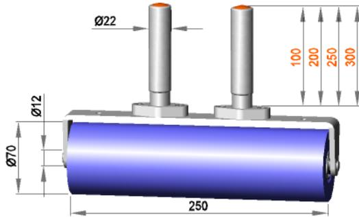
Fixed roller assembly with roller **R 12 / 250 / 70 / S50R**
