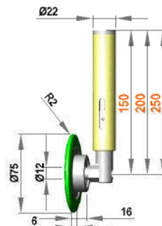
**Spring-mounted roller assembly with roller RRL 12 / 18 / R5 / S30B**
