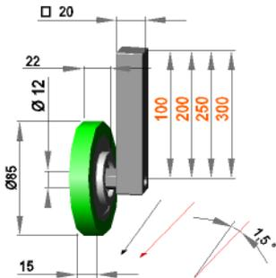
Guide roller assembly 1,5° left with roller F 12 / 15 / 85 / AL
