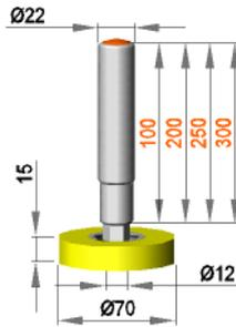
**Fixed roller assembly with roller R 12 / 15 / 70 / S90Gr**
