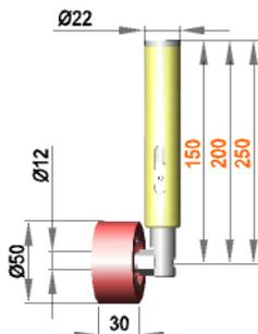
**Spring-mounted roller assembly with roller R 12 / 30 / 50 / S70G**
