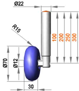
**Fixed roller assembly with roller RR12 / 30 / R15 / S50R**
