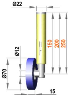
Spring-mounted roller assembly with roller R 12 / 15 / 70 / S50R
