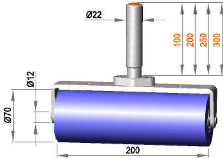
Fixed roller assembly with roller **R 12 / 200 / 70 / S50R**
