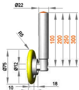
**Fixed roller assembly with roller RRL 12 / 18 / R5 / S90Gr**
