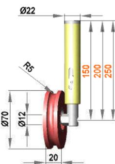
Spring-mounted roller assembly with roller NR12 / 20 / R5 / S70G
