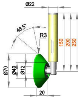
Spring-mounted roller assembly with roller FR12 / 20 / R3 / AL
