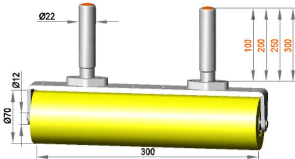
Fixed roller assembly with roller **R 12 / 300 / 70 / S90gr**
