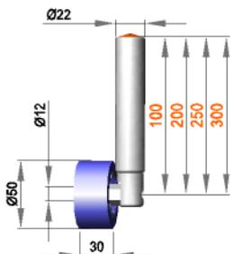
**Fixed roller assembly with roller R 12 / 30 / 50 / S50R**
