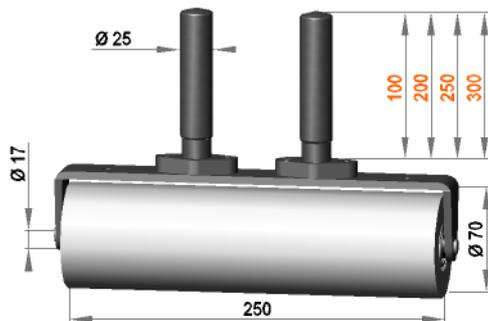
Roller assembly Ø25 with press roller **R 17 / 250 / 70 / PO**
