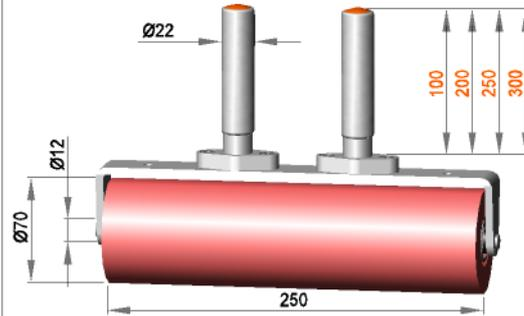
Fixed roller assembly with roller **R 12 / 250 / 70 / S70G**
