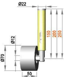
**Spring-mounted roller assembly with roller R 12 / 50 / 70 / PO**
