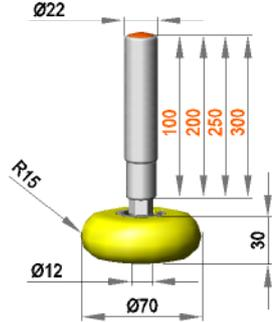
**Fixed roller assembly with roller RR12 / 30 / R15 / S90Gr**
