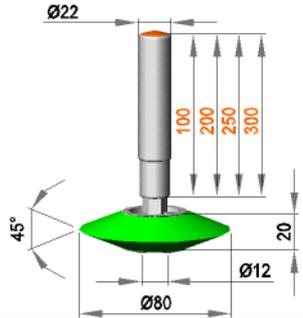
**Fixed roller assembly with roller ER 12 / 20 / 45 / AL**
