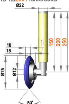
Spring-mounted roller assembly with roller ERL 12 / 18 / 80 / S50R
