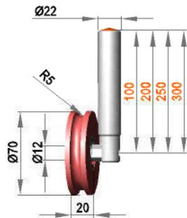
**Fixed roller assembly with roller NR12 / 20 / R5 / S70G**
