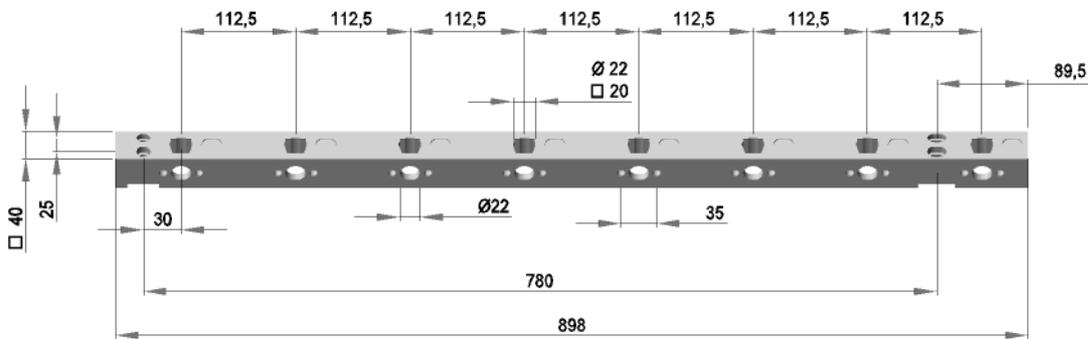
Tool head for height adjustment
