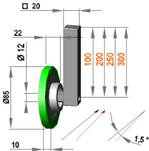
Guide roller assembly 1,5° right with roller F 12 / 10 / 85 / AL
