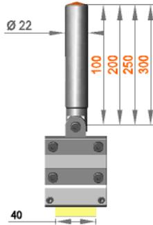
Fixed assembly with felt holder FH/G/60
