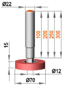
**Fixed roller assembly with roller R 12 / 15 / 70 / S70G**
