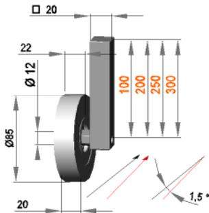
Guide roller assembly 1,5° right with roller F 12 / 20 / 85 / PO
