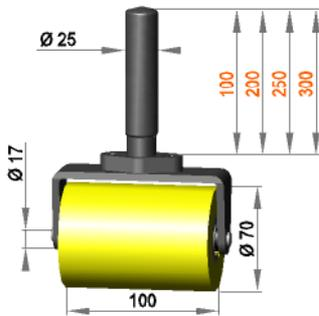
Roller assembly Ø25 with press roller **R 17 / 100 / 70 / S90Gr**
