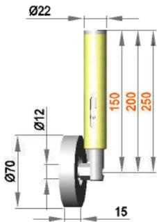
Spring-mounted roller assembly with roller R 12 / 15 / 70 / PO
