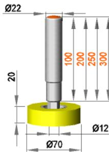
**Fixed roller assembly with roller R 12 / 20 / 70 / S90Gr**
