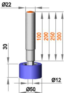
**Fixed roller assembly with roller R 12 / 30 / 50 / S50R**
