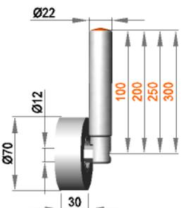
**Fixed roller assembly with roller R 12 / 30 / 70 / PO**
