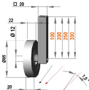
Guide roller assembly 1,5° left with roller F 12 / 20 / 85 / PO
