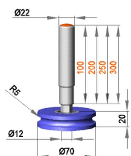
**Fixed roller assembly with roller NR12 / 20 / R5 / S50R**
