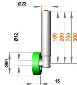
**Fixed roller assembly with roller R 12 / 15 / 50 / AL**
