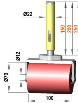
Spring-mounted roller assembly with roller **R 12 / 100 / 70 / S70G**
