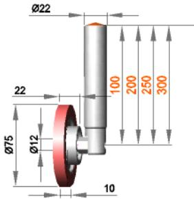
**Fixed roller assembly with roller R 12 / 10 / 75 / S70G**
