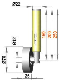
Spring-mounted roller assembly with roller R 12 / 25 / 70 / PO
