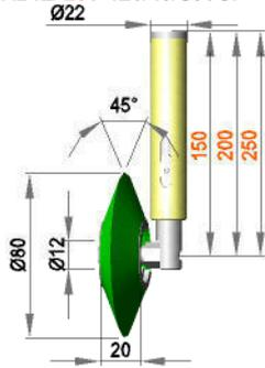
Spring-mounted roller assembly with roller ER 12 / 20 / 45 / AL
