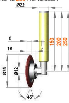
Spring-mounted roller assembly with roller ERL 12 / 16 / 45 / S70G
