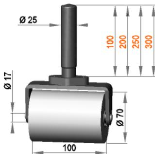
Roller assembly Ø25 with press roller **R 17 / 100 / 70 / PO**
