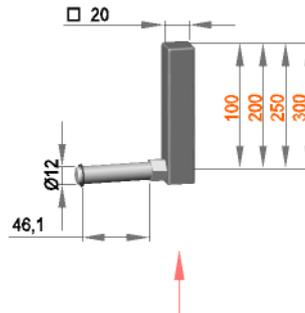
The low gradient of 1.5° set the guide roller obliquely. So the profile is pressed with slight pressure. **This right version must be arranged with the left version.**
