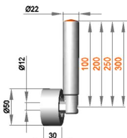
**Fixed roller assembly with roller R 12 / 30 / 50 / PO**
