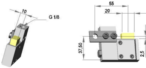
Felt holder, mounted below, right-side version, rigid design
