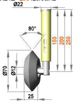
Spring-mounted roller assembly with roll ER 12 / 25 / 80 / PO
