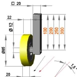
Guide roller assembly 1,5° left with roller F 12 / 20 / 85 / S90Gr
