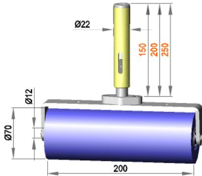
Spring-mounted roller assembly with roller **R 12 / 200 / 70 / S50R**
