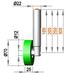
**Fixed roller assembly with roller R 12 / 25 / 70 / AL**
