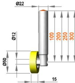
**Fixed roller assembly with roller R 12 / 15 / 50 / S90Gr**
