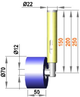
**Spring-mounted roller assembly with roller RB 12 / 50 / 70 / S50R**
