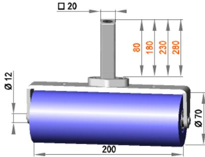
Square roller assembly with roller R 12 / 200 / 70 / S50R
