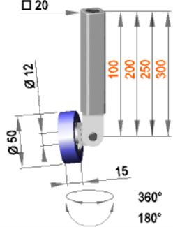
**Universal roller assembly with roller R 12 / 15 / 50 / S50R**
