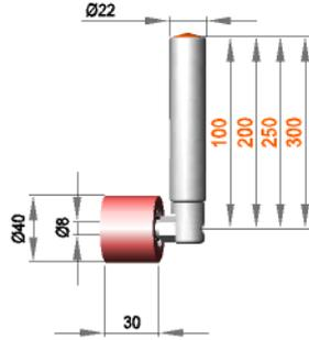
**Fixed roller assembly with roller R 8 / 30 / 40 / S70G**
