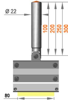
Fixed assembly with felt holder FH/G/100
