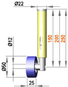
**Spring-mounted roller assembly with roller R 12 / 25 / 50 / S50R**
