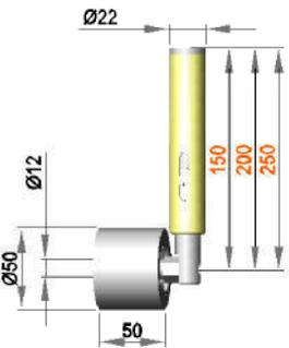
**Spring-mounted roller assembly with roller RB 12 / 50 / 50 / PO**
