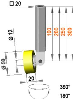
**Universal roller assembly with roller R 12 / 20 / 50 / S90Gr**
