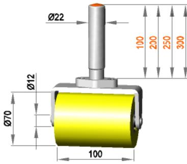
Fixed roller assembly with roller **R 12 / 100 / 70 / S90Gr**
