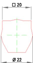
The tool heads are designed for tool holders with a diameter of 22mm and for a 20mm square cross section. The clamping element can be used for faster changing of individual tool holders.
