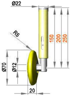
Spring-mounted roller assembly with roller RR12 / 20 / R5 / S90Gr
