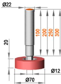
**Fixed roller assembly with roller R 12 / 20 / 70 / S70G**
