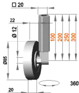
**Swiveling guide roller assembly with roller F 12 / 20 / 85 / PO**
