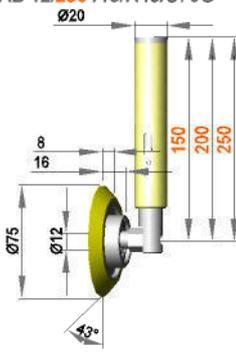
Spring-mounted roller assembly with roller ERL 12 / 16 / R43 / S90Gr
