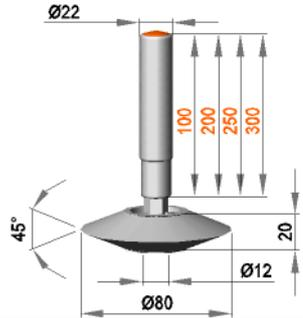
**Fixed roller assembly with roller ER 12 / 20 / 45 / PO**
