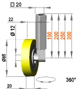
**Swiveling guide roller assembly with roller F 12 / 20 / 85 / S90Gr**
