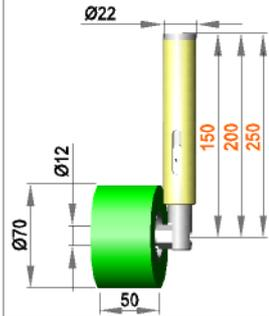
**Spring-mounted roller assembly with roller R 12 / 50 / 70 / AL**
