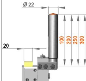
Fixed assembly with felt holder FH/G/20
