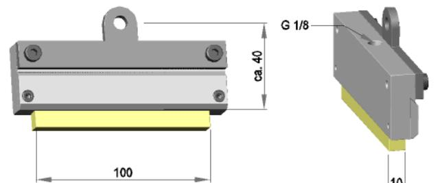
Felt holder, mounted below, left-side version, rigid design
