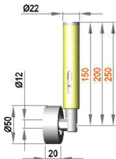
Spring-mounted roller assembly with roller R 12 / 20 / 50 / PO
