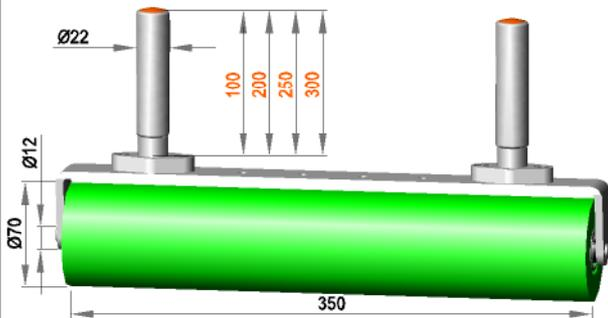
Fixed roller assembly with roller **R 12 / 350 / 70 / AL**
