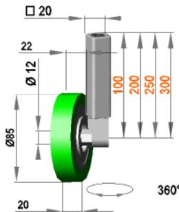
**Swiveling guide roller assembly with roller F 12 / 20 / 85 / AL**
