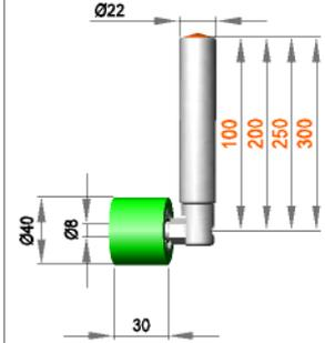
**Fixed roller assembly with roller R 8 / 30 / 40 / AL**
