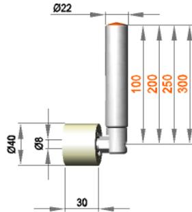
**Fixed roller assembly with roller R 8 / 30 / 40 / ST**
