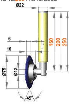
Spring-mounted roller assembly with roller ERL 12 / 16 / 45 / S50R
