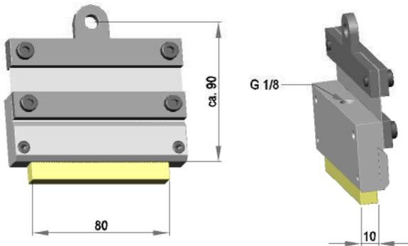
Spring-mounted felt holder, 100mm, mounted top
