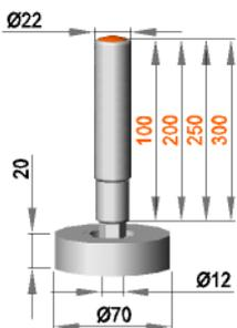
**Fixed roller assembly with roller R 12 / 20 / 70 / PO**
